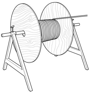
A simple to use cable payoff system consisting of two 'A' frames with a centre axle.
