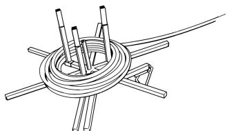
Easy method of uncoiling loose coils cable, hose, flexible tubing, rope and wire rope.
