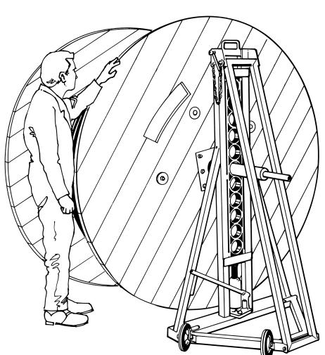
Maximum drum size Diameter: 2600mm Width: 2000mm
